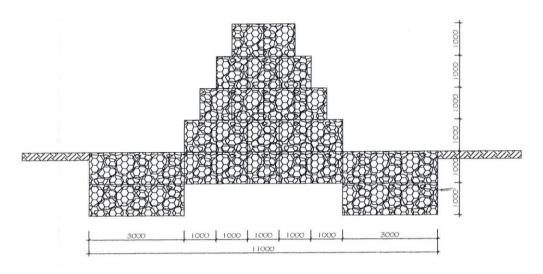
Figure 4: Cross section of a spur design in Chitwan showing substantial groundwork Illustration: Practical Action Nepal.
