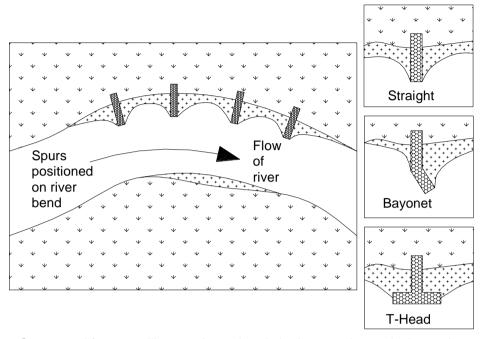
Figure 3: Spurs used for controlling erosion at bends in rivers and spur design options.
