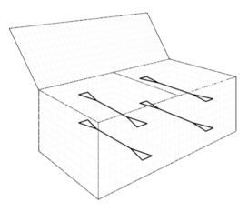
Figure 11: Cross links with wire Illustration: Practical Action / Neil Noble
